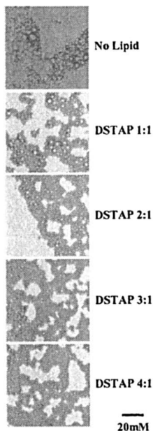
Figure 3. Effect of cationic lipid concentration on particle size. Particles were generated using different concentrations of DSTAP, and particle size was analyzed using light microscopy.
